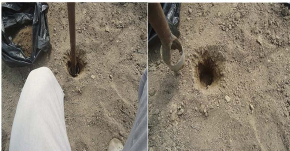
Figure 2. Illustration of use of hand corer for soil sampling.
