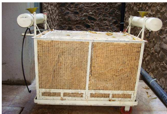
Figure 2. Photographic view of evaporative cooler.
