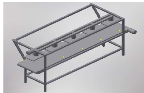
Fig 1. Frame of the de-lidding machine.
