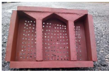
Fig 3. Tray with double cone shape air flow
